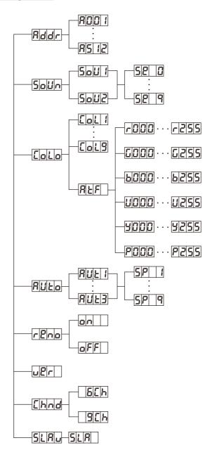
Addr - DMX Address Setting via control board
