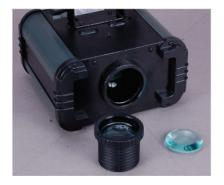
Unscrew and remove the focus barrel. Using your thumb, gently push the lens outward until it pops out.
