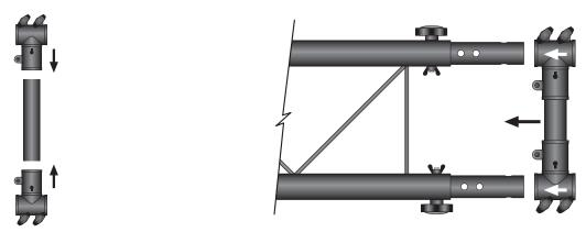
Assemble the second half of the Truss I-Beam by inserting one end of the second Truss I-Bar onto the I-Beam connectors that were installed in the previous step. Insert the connector knobs through the I-Beam and fasten with the wing nuts.
