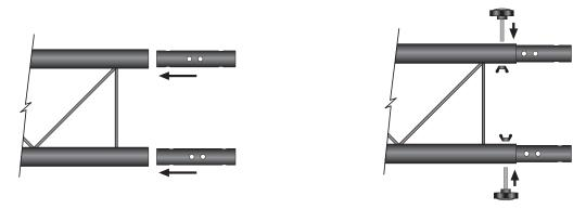
Assemble the Support Rod by inserting a Slide Mount T-Collar onto each end of the Support Rod. Slide the assembled Support Rod onto the I-Beam connectors.
