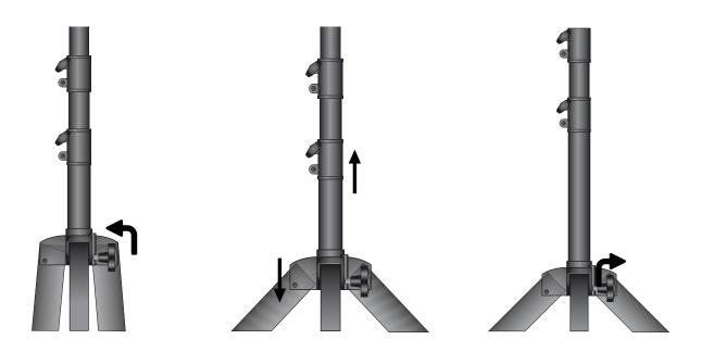
Loosen Knob C by turning it counter clockwise. Extend the inner pipe to the desired height and insert the safety pin through the stopper holes in the inner pipe. Secure and tighten Knob C by turning it clockwise. Repeat this process to set the desired height for the center post as well.
