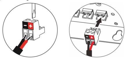
DarkFX Strip 510 is wired to output terminal of DarkFX Drive 4. Each output terminal can connect one DarkFX Strip 510 fixture.
