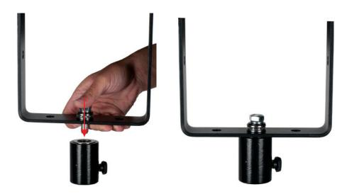
Align the mounting hole of the fixture yoke with the threaded hole of the Locking Ferrule on the FS Pan Glide, then insert and tighten the silver hex bolt and its washer assembly (see Washer Assembly Stack Sequence on next page). Be careful to not drop or lose the washers in the process. The fixture is now attached to the FS Pan Glide.
