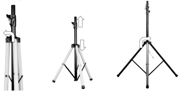
Loosen Knob B by turning it counter clockwise. Extend the center post to the desired height and insert the safety pin through the stopper holes in the center post. Secure and tighten Knob A by turning it clockwise.
